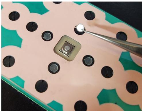
The 4 directional buttons require a dot sticker attached to the center **AFTER** replacing the backlight film over the membrane keypad repair.
